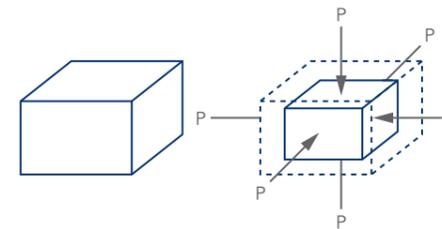
Rockdelta elastic mats possess a uniquely high degree of volume compressibility with a Poisson's Ratio of almost zero.
