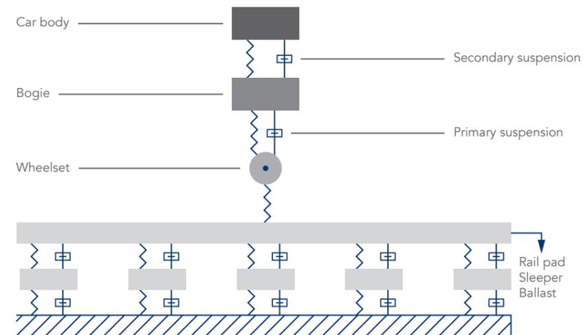
Now imagine a railway system situation. The running train generates a force which is transmitted from the top of the rail to the elements below the track superstructure. To limit the effect of those forces, a spring (elastic material or isolator) should be inserted to absorb mechanical energy.
