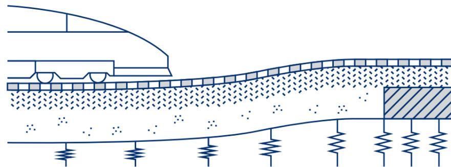
The easiest way to build transition zones is by placing elastic elements just below the ballast bed or slab track. Creating transition zones with other methods, such as by varying the sleeper spacing or the fastener stiffness is complicated and requires a high degree of precision. By simply changing the stiffness of the elastic mat, the overall stiffness of a section of track can be easily adapted.
