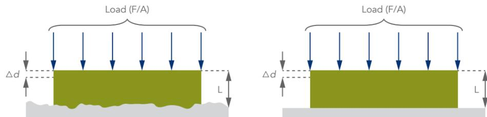
The diagram above on the right shows a perfectly leveled sub-grade while the left diagram shows an uneven sub-grade. Rockdelta elastic mats can be installed in both situations with no change in Insertion Loss.
