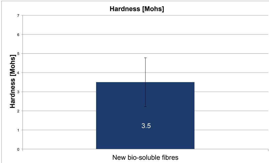
Measured values of hardness for new developed stone fibres
